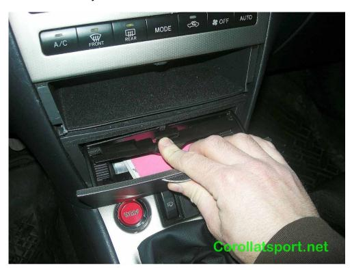
Step 2 - lift up and put aside the cover around the gearstick
