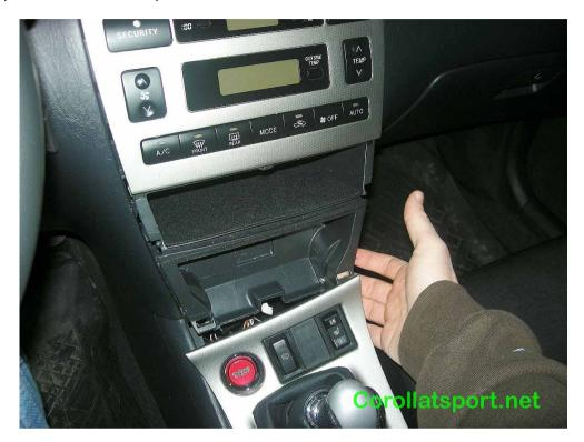
Step 4 - grab on each side of the ac control display and pull the console out
